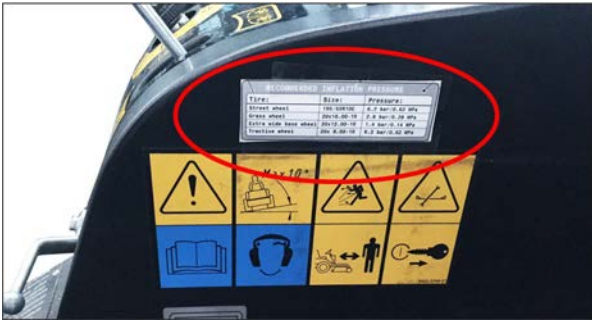
Figure: Label in the driver cabin with recommended tyre pressures
